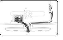
**5** Fasten the 1 screw on the cover(B).
